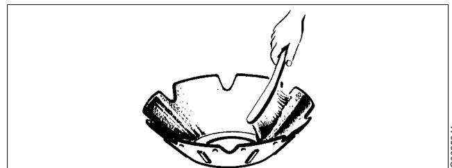
Clean the discs with a soft brush
