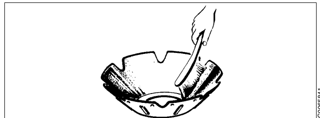
Clean the discs with a soft brush
