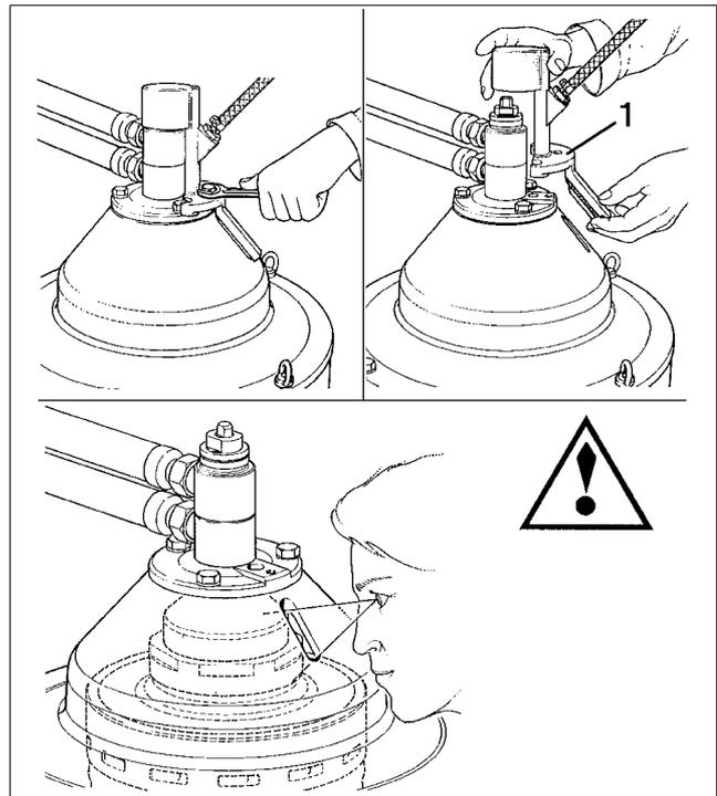
2. Unscrew nut (2) clockwise and lift off inlet and outlet housings (3, 4) together with the connecting hoses. When removing the connecting hoses, do not drop the washer.
