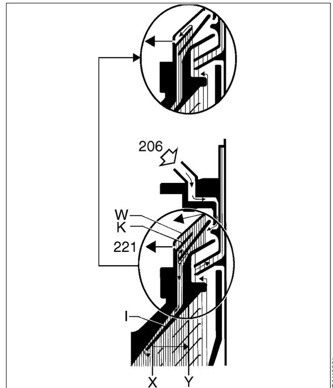
*Principle of liquid seal and displacement water in purification*
