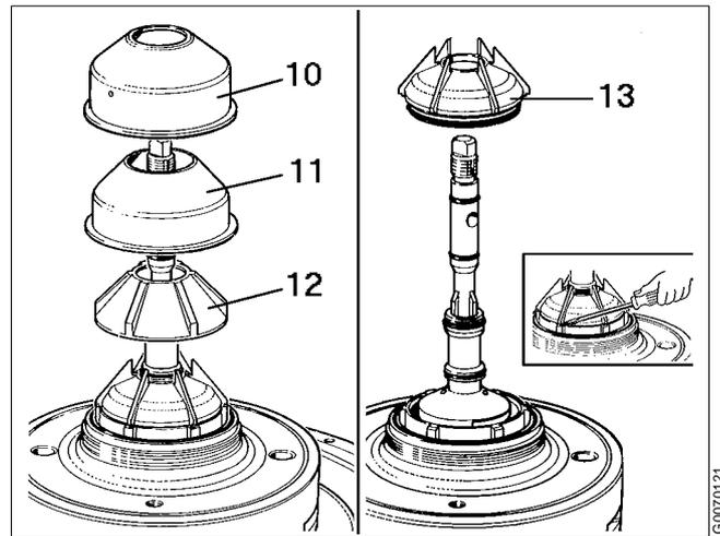
6. Carefully prise loose paring chamber cover (13) by using a screwdriver. Lift off the paring chamber cover.
