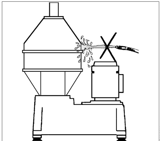
*Never wash down a separator with a direct water stream or spray*
