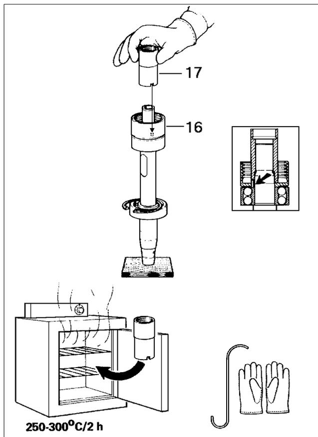
5. Check that the radial hole ( $\phi$  1 mm) in the pump sleeve (18) is clean, and fit the pump.
