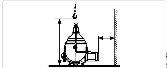
*Suitable space must be obtained for the maintenance work*
