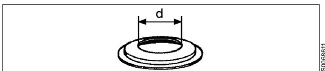
*Gravity disc diameter sets the oil/water interface*
