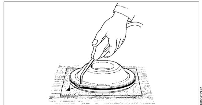
Removal of seal ring on sliding bowl bottom
