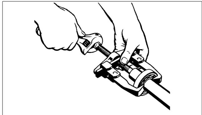
For bearings where no driving-off sleeve is included in the tool kit, use a puller when removing bearings
