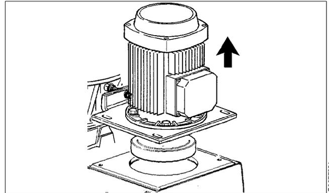
6. Remove snap ring (9), cover (8) and friction elements (7).
