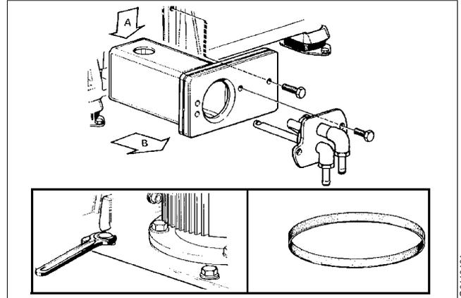
5. Remove the electric motor complete with the friction coupling and motor adapter.
