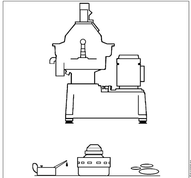
*Remove the bowl if the separator is left at standstill for more than one week*
