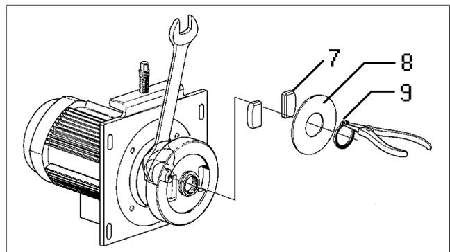
7. Degrease and clean the contact surfaces of frame and motor adapter. Lubricate the contact surfaces with Molykote 1000 paste. Then fit the electric motor with adapter and friction coupling in position.
