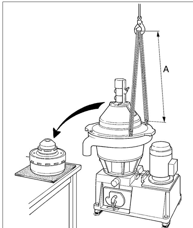
A minimum 750 mm distance between lifting eye and hook. Use a lifting hook with catch.
