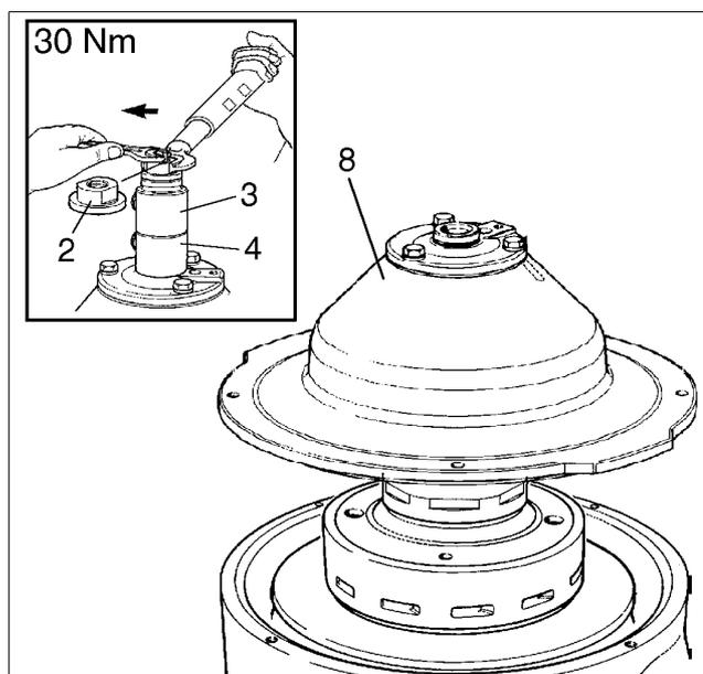
20. Make sure that the gasket on the safety device is in position. If not, glue with Loctite 407.
