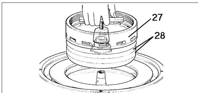
18. Ease the bowl body off with the central screw of the tool. If necessary, knock on the handle.
