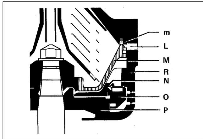
*Sludge discharge mechanism*
