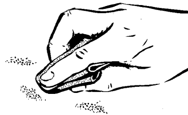
Polish corrosion marks to prevent further damage
