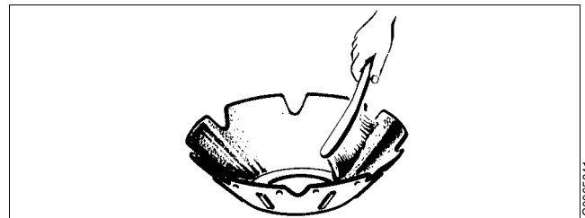
Clean the discs with a soft brush
