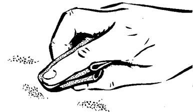
Polish corrosion marks to prevent further damage.
